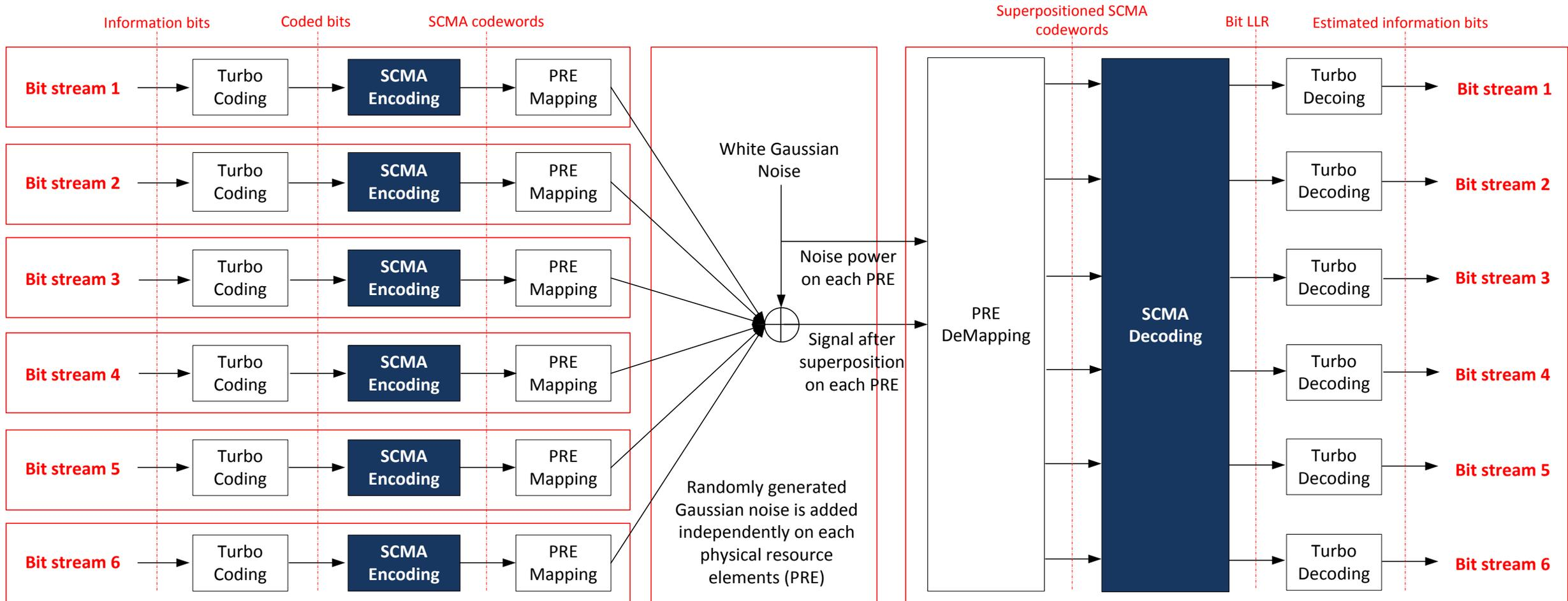
\* Turbo coding and decoding can be replaced by other forward error correction (FEC) channel coding/decoding modules.
